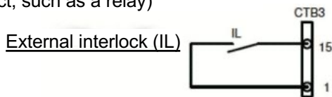
Connection diagram 5. (When used by connecting to a contact, such as a relay)
